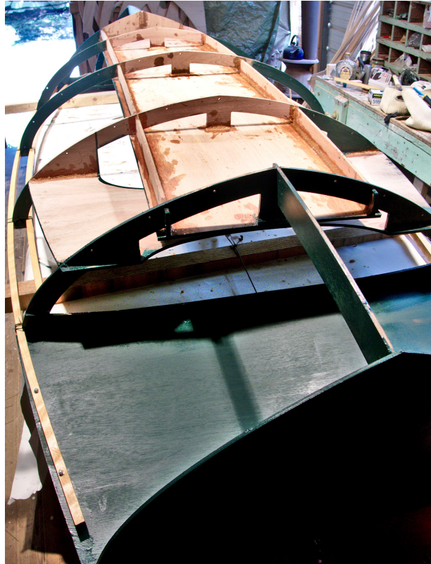
Figure 4.3. Plywood frame, preparing to paint the underside
