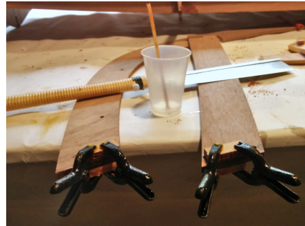
(b) Front and back keel parts with sticks to increase width
