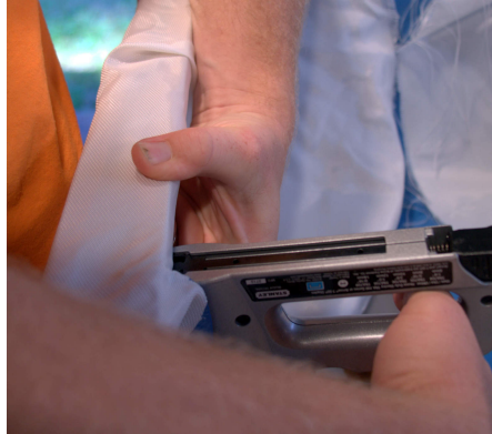
(a) Stapling skin to underside of the gunwales
