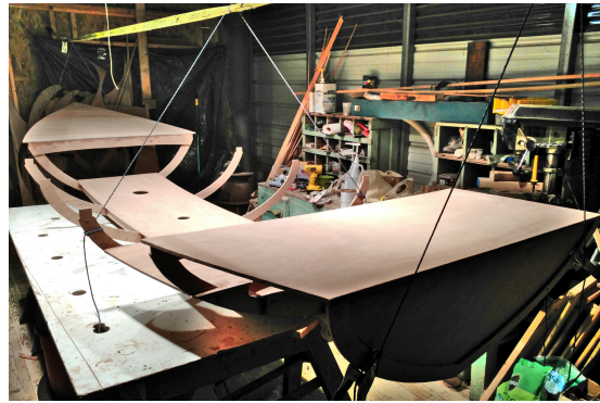
(b) Supporting the stern (and bow) with ropes
