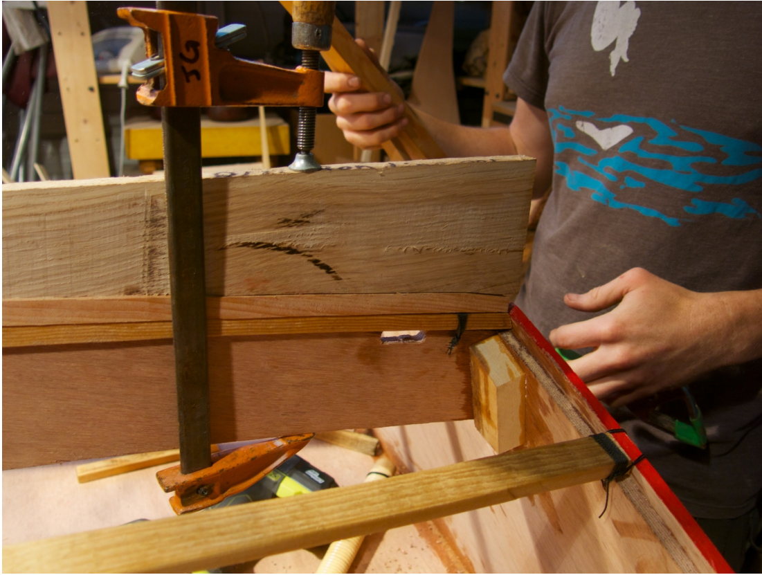
Figure 7.1. Placing the skeg ahead of time, cutting recesses for keel bolts
