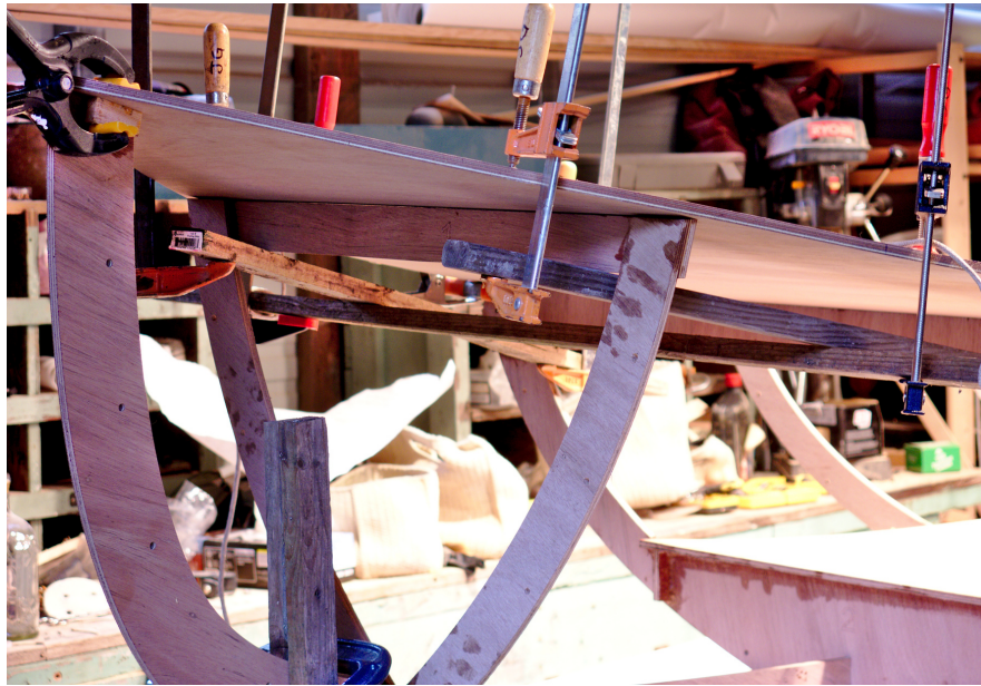
(a) Creating a bend using external boards and clamps
