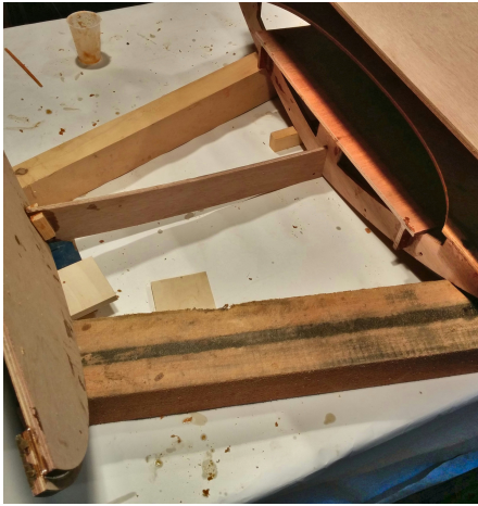
(a) Supporting the stern with boards
