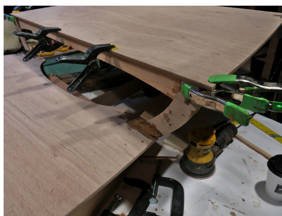
(b) Getting the clamps right for the aft deck and seat
