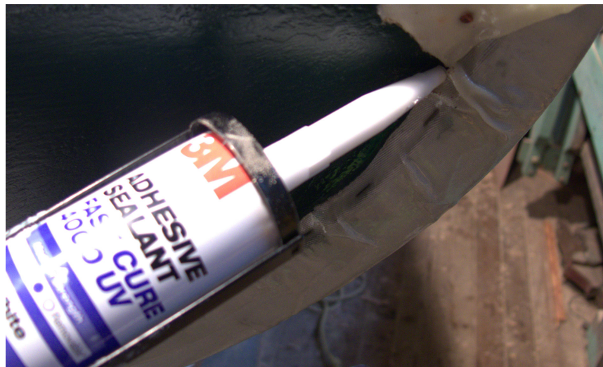
Figure 6.11. Sealing the transom
