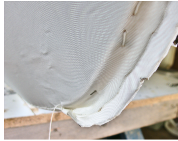
(b) Trimming edges
