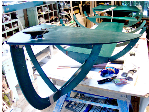
Figure 4.2. Plywood frame, the top sanded and painted
