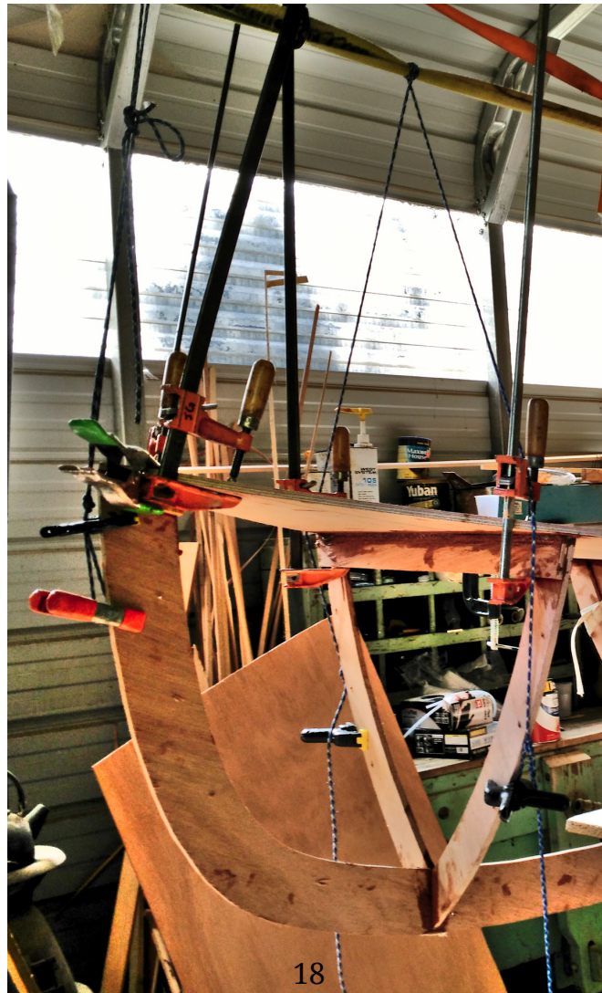
(b) Creating a bend using clamps and rope
