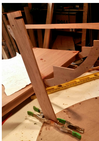
(a) Gluing transom to the keel
