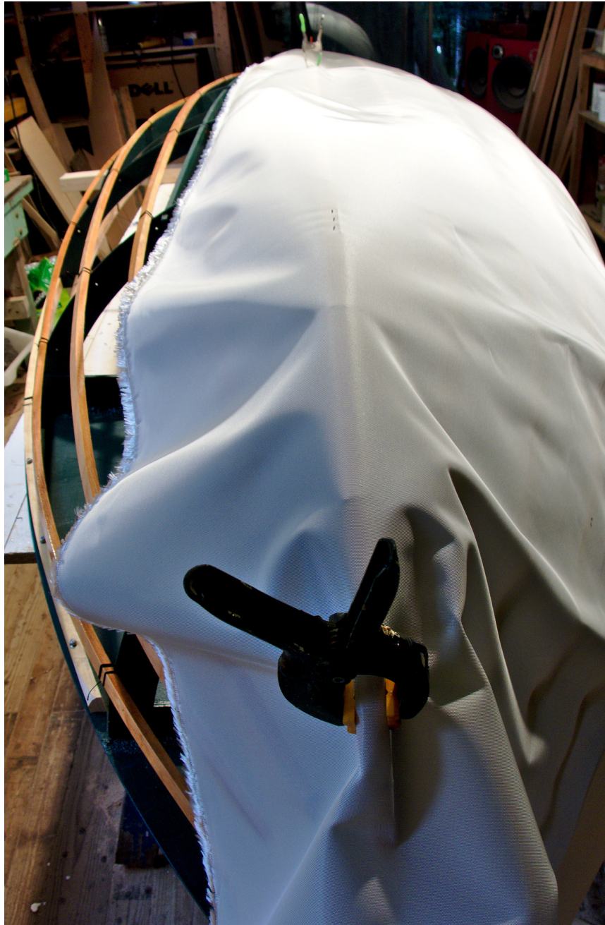
Figure 6.1. Draping the skin over the frame
