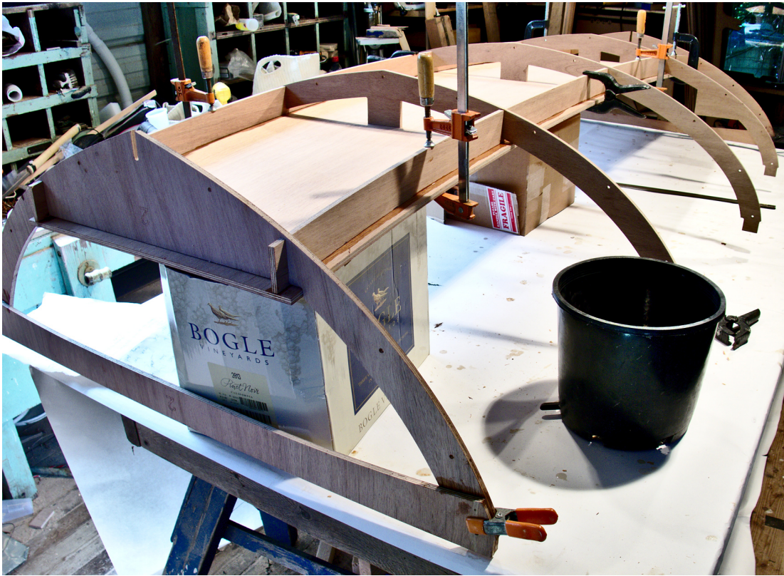
Figure 3.2. Test fitting the frames and spine for the middle of the boat
